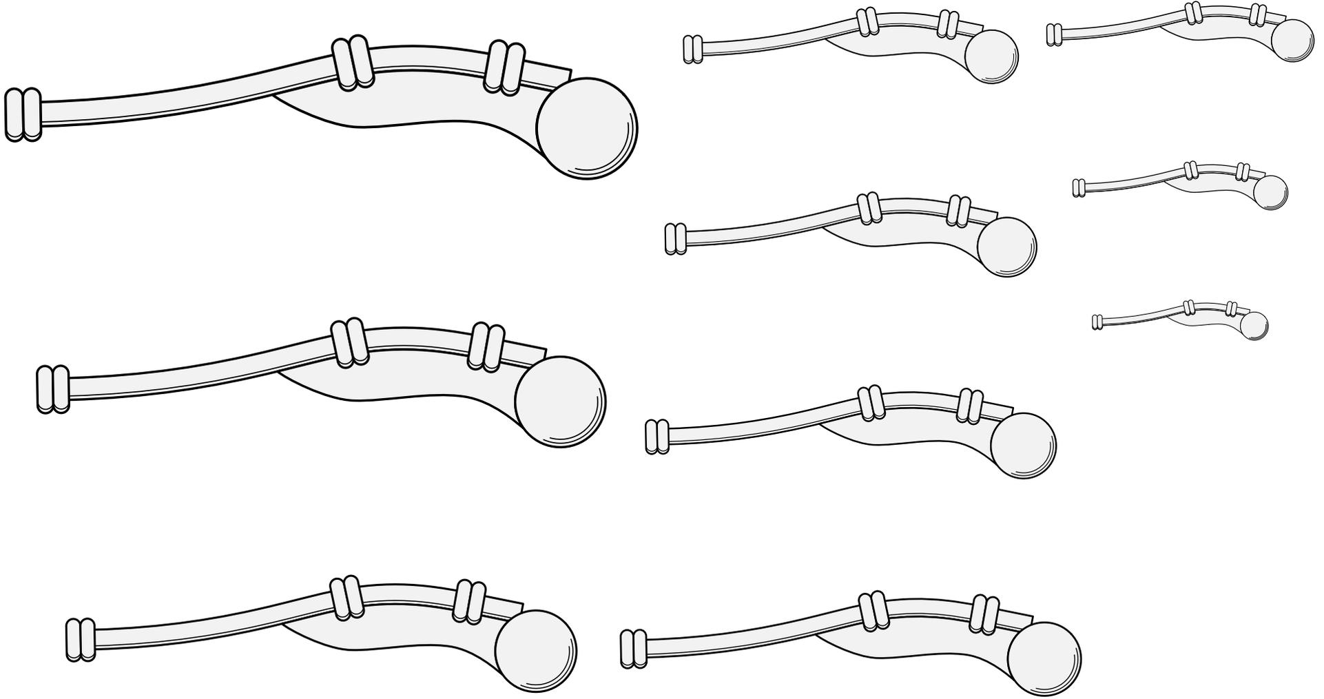
A whistle used to command the attention of a ship's crew, with a metal pipe leading to an metal sphere.
