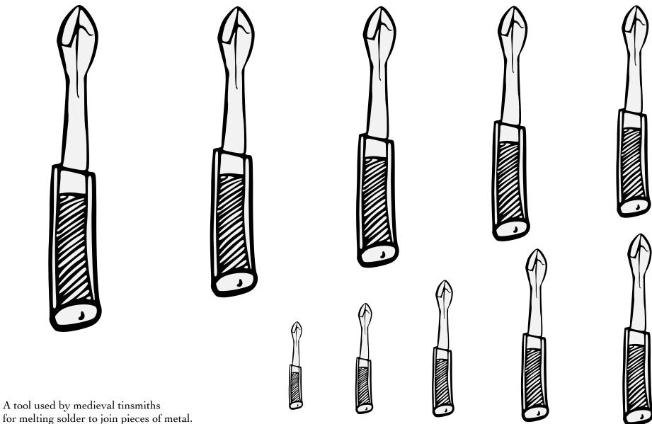
for melting solder to join pieces of metal.
