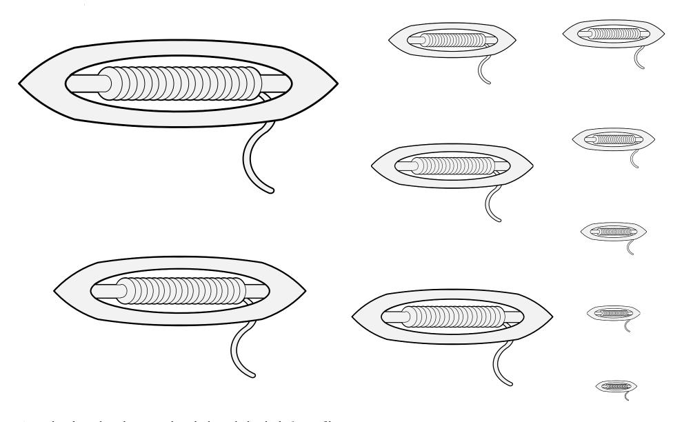
An enclosed spool used to carry threads through the shed of warp fibers.
