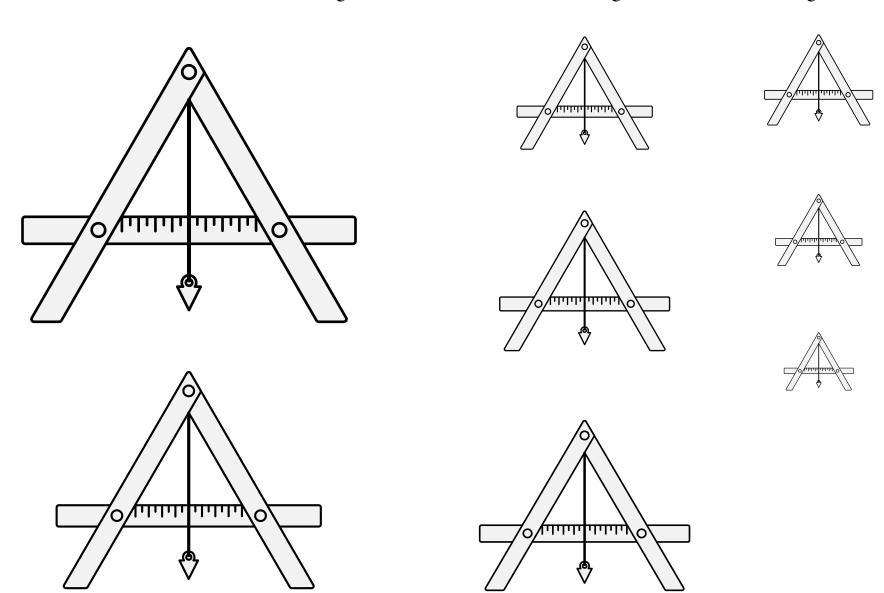
A builder's tool for ensuring surfaces are horizontal or vertical.
