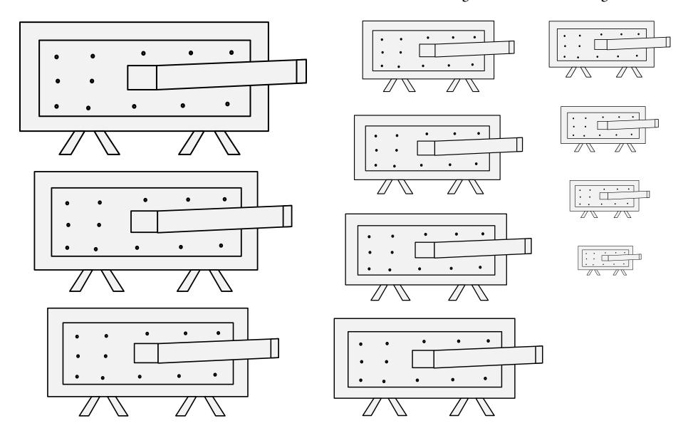
A tool for crushing hemp stalks to separate the fibers for making fabric. Also called a "hemp-bray."
