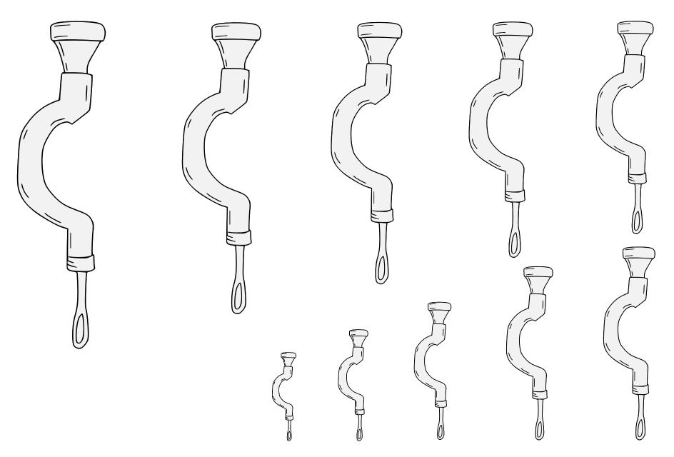
A woodworking tool used for making holes, with an offset hand crank for rotary power.
