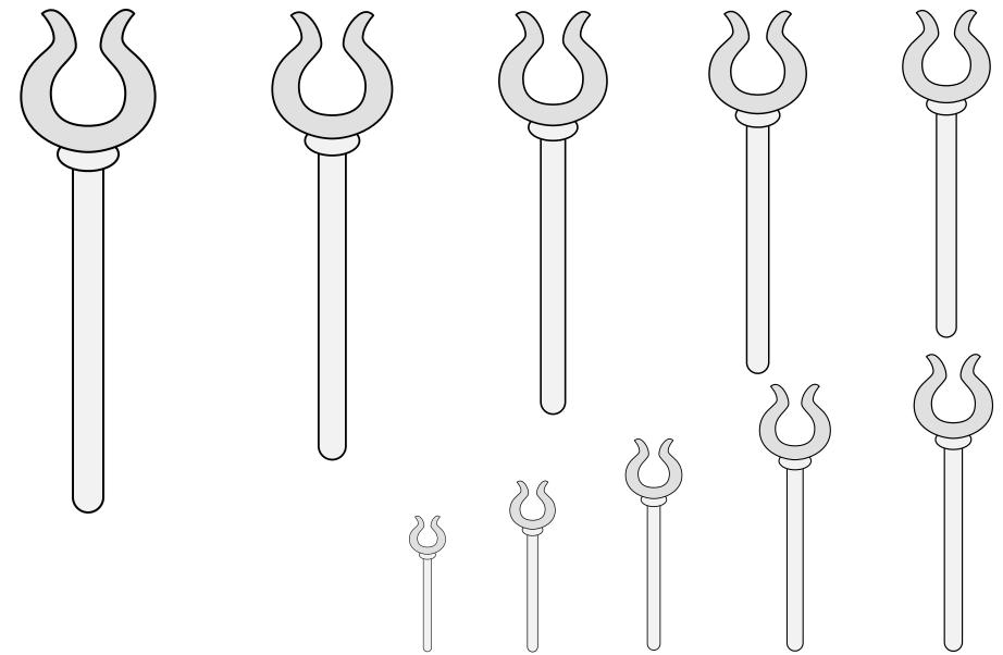
A pivoting pin with a forked head used to secure oars to the side of a boat.
