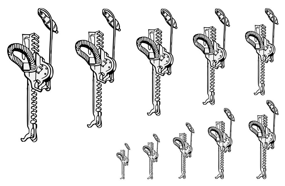
A geared mechanism used to span a crossbow.
