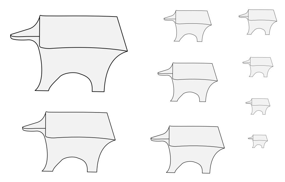
A solid base used for shaping metal.
