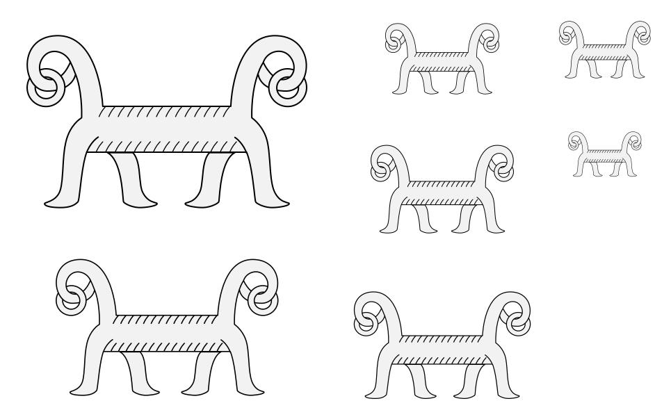
A metal structure used to hold firewood in place while it burns.
