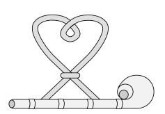
A whistle used to command the attention of a ship's crew, with a metal pipe leading to an metal sphere.
