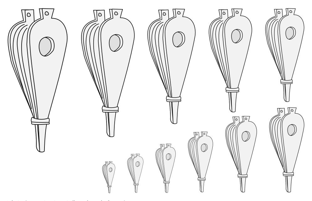
A device for pumping air, typically used to stoke fires or forges.
