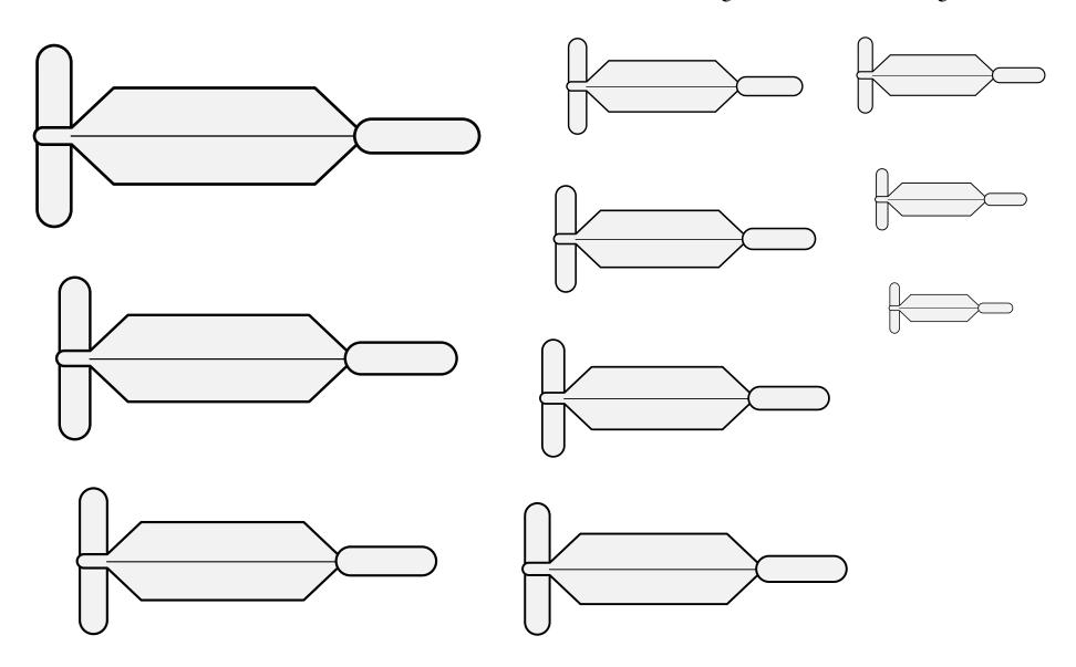
A long straight-edged knife with two handles, used to trim the hair off of hide when making leather.
