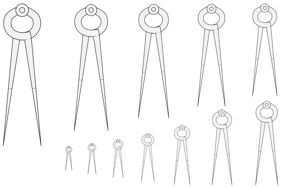
Two pins joined by a pivot used for measurement when drawing or building.
