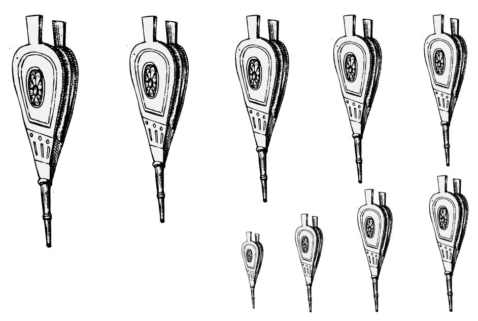
A device for pumping air, typically used to stoke fires or forges.
