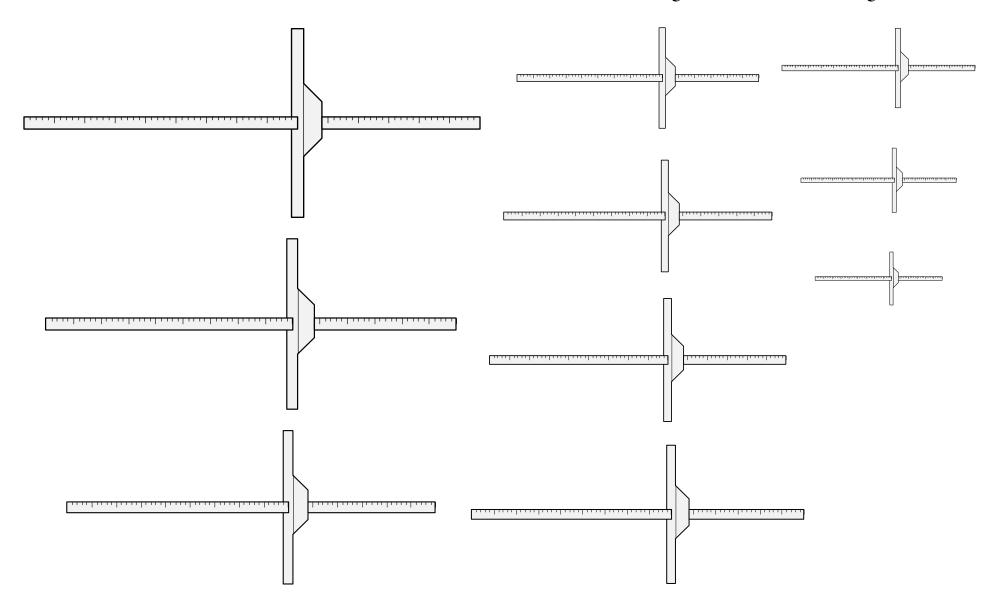
A tool used by surveyers and astronomers to measure angles to distant objects.
