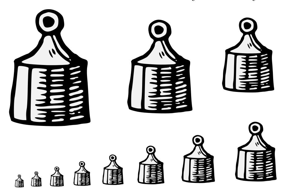
A lead weight, to be attached to a cord for use as a plumb line or sounding line.
